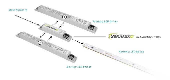
The sheer simplicity of the Xeramix R device is what makes it so effective. The power flows to the primary LED driver via the internal relay, which is energised by the primary driver's output. When the primary LED driver output fails, it will no longer power the relay coil, switching the mains power to the backup driver. A small external indicator shows if this has occurred and the backup driver is engaged.
