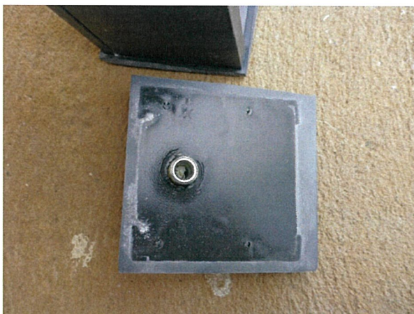
Inspection after IP6x test
