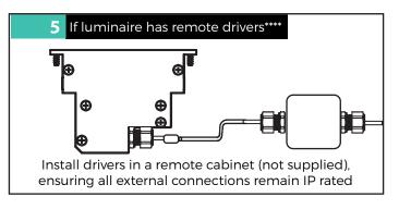
Connect electrical cables ensuring that the cable lengths are all the same and do not exceed the maximum rated length
